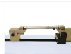
zero setting and calibration of tubular inside micrometers
