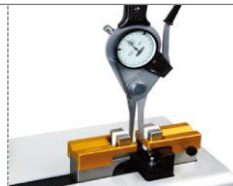
zero setting and calibration of internal/external snap gauges
