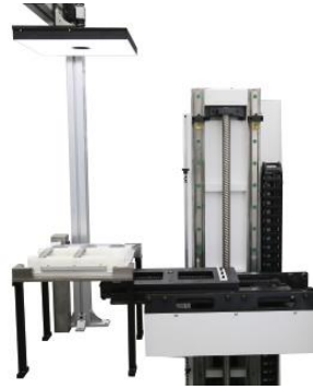
The palletizing elevator automatically conveys the workpiece pallets to the vision positioning station
