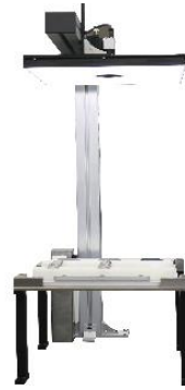
The vision positioning station automatically verifies the workpiece placement position
